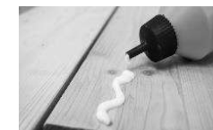
Joint with wood glue or PVA
